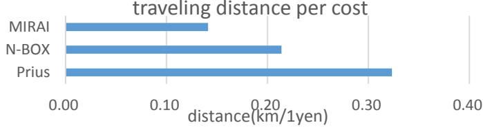
Hydrogen fuel cell vehicle is still inferior to gasoline car, especially its "cost performances" and hard to say it meets the demand.
